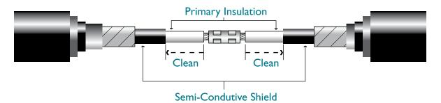
3. Apply LPS cable cleaner to a clean lint-free cloth and remove all the remaining semi-conductive and conductive particles on the primary insulation by wiping from the insulation edge back toward the semi-conductive shield. Wipe the primary insulation dry with a lint-free cloth.
